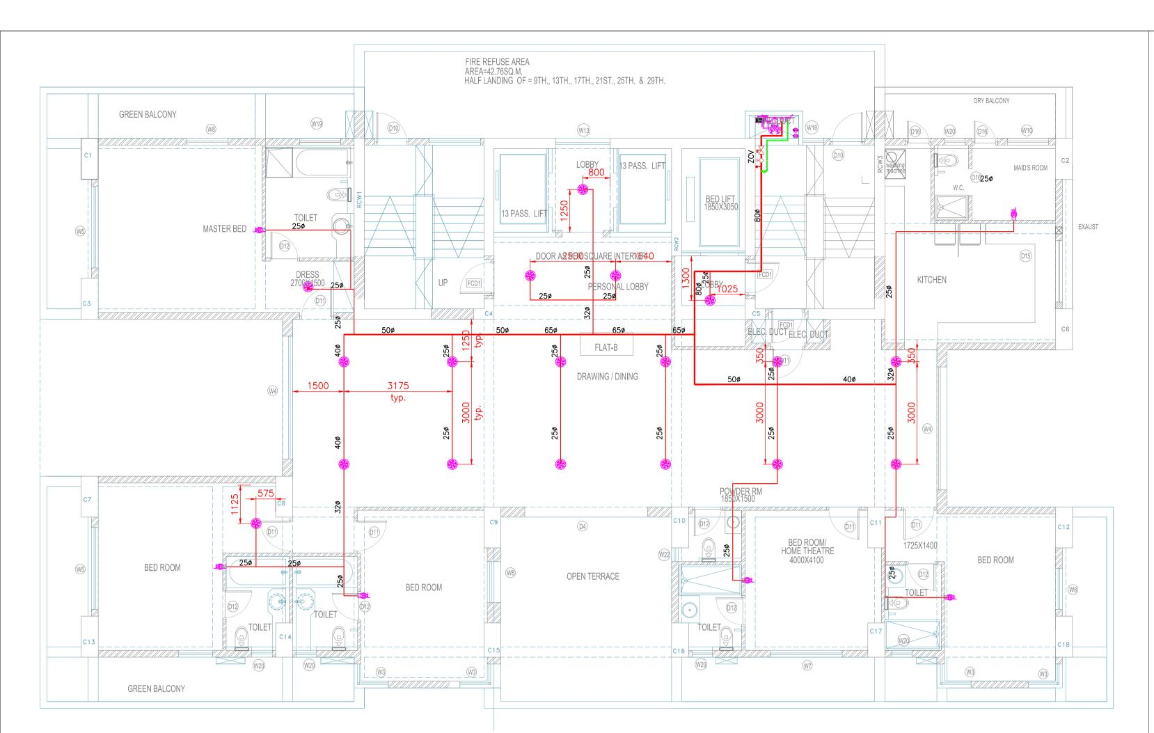
SLEEVES @ 10TH FLOOR STRUCTURE FIRE FIGHTING SLEEVE LAYOUT SCLE 1:75
